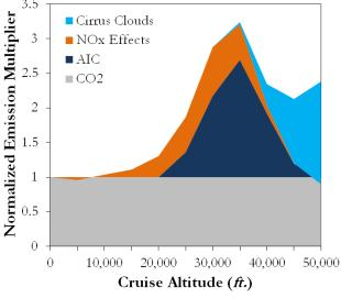
Fig. 70 Environmental multiplier vs. altitude
