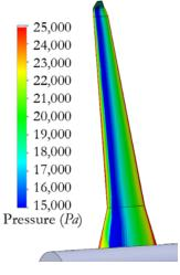
Fig. 19 Pressure contours adjacent to the upper surface of the wing
