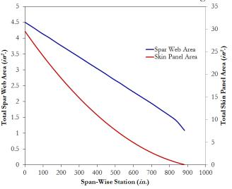
*al*<sup>70</sup>. In conjunction with the trade study **Fig. 63 Total spar and skin panel area vs. span-wise station** presented in Section 4.4, a wing planform with an AR of 14.1 was confirmed to be below the flutter limits set by the previously mentioned publications and, therefore, demonstrated an achievable structural solution with integrity. Figure 64 presents the results of this parametric study.
