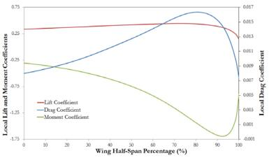
Fig. 60 Lift, drag, and moment coefficients vs. wing half span %
