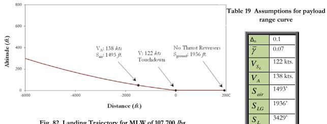
Fig. 82 Landing Trajectory for MLW of 107,700 lbs.
