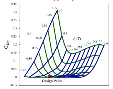
Fig. 12 Forebody Wave Drag Coefficient Vs. Cruise Mach Number ( $M_o$ ) and Bluntness Ratio (d/D). The bluntness ratio corresponding to the lowest wave drag coefficient was chosen as the design point.
