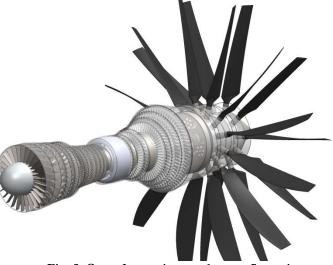
Fig. 5 Open fan engine, pusher configuration
