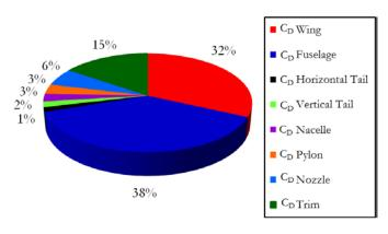
Fig. 24 Drag breakdown at cruise.
