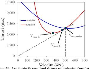
Fig. 79 Available & required thrust vs. velocity (cruise)
