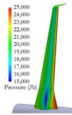
Fig. 20 Pressure contours adjacent to the lower surface of the wing
