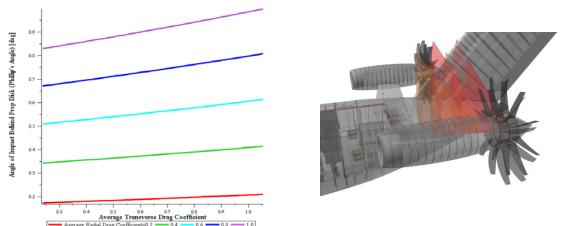
Fig. 36 Impingement angle as a function of radial and transverse drag coefficients, for takeoff conditions(left) CAD illustration of blade impingement angles(right)
