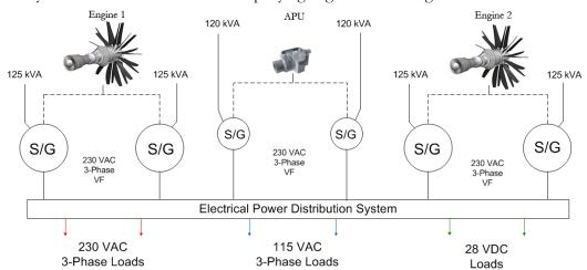
Fig. 45 Electrical power generation architecture. S/G denotes starter/generator units installed on the engines and APU. V/F denotes variable frequency.
