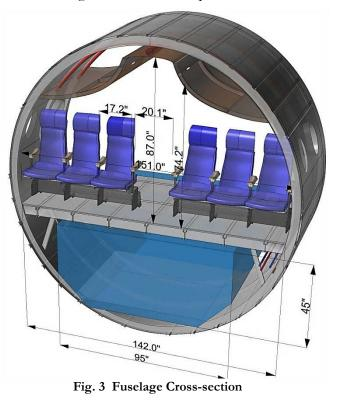
are designed to provide 2.7  $ft^3$  of volume for the passengers in a seating arrangement with a seat pitch of 32". Egret has the capability of carrying a maximum of 1,410  $ft^3$  of containerized cargo and 180  $ft^3$  of bulk cargo on the lower deck.
