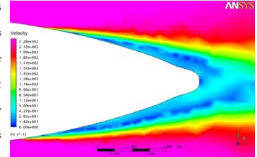
Fig. 34 CFD transient analysis performed using CFX Package showing boundary layer thickness around fuselage tailcone at takeoff.
