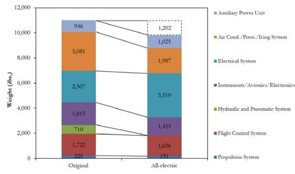
Fig. 57 Egret's weight adjustments due to all-electric architecture. Note that net weight reduction is indicated above the right hand weight column.
