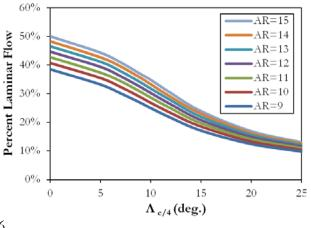
Fig. 16 Extent of Laminar Flow vs. Quarter Chord Sweep of the wing.
