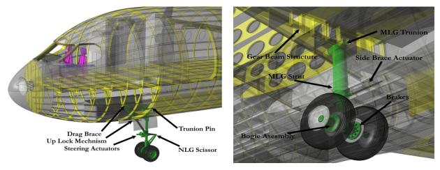
Fig. 48 Nose landing gear
