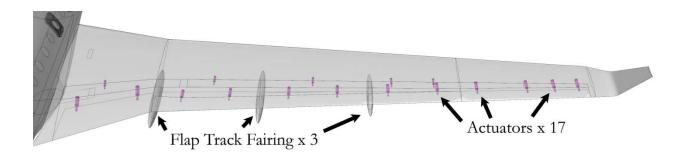
Fig. 47 Location of control surface actuators and flap track fairings
