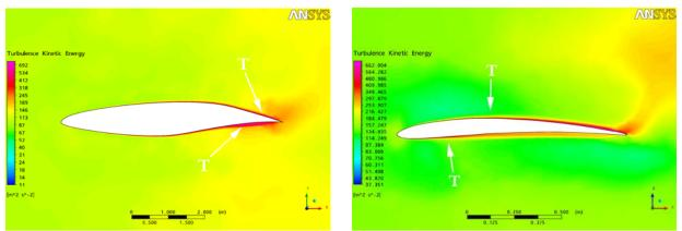
Fig. 14b Turbulence Kinetic Energy for wing root airfoil Fig. 15b Turbulence Kinetic Energy for wing tip airfoil
