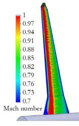
Fig. 18 Mach number contours adjacent to the upper surface of the wing
