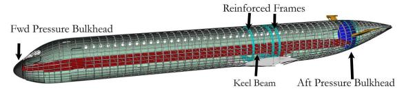
Fig. 65 Fuselage Structure
