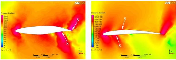
Fig. 14a Pressure Gradient for wing root airfoil
