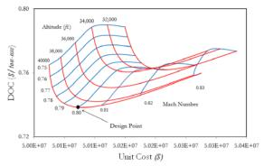
Fig. 86 DOC vs. unit cost for various initial cruise altitudes and Mach numbers, at a range of 1,200 *nm.* for a production run of 500 aircraft..
