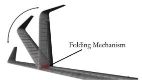
Fig. 55 The operation of the folding mechanism
