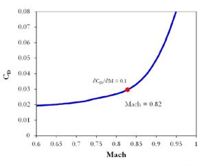
Fig. 25 Result of drag divergence analysis on Egret indicating a  $M_{DD}$  of 0.82, according to the criteria of  $\partial C_D / \partial M$  of 0.1.
