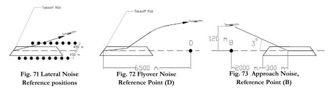
ICAO Chapter 4 also cites the maximum value of the acceptable noise for each of the described reference measurement positions, and allows a cumulative deviation of 3 *dB* from the **Table 14 Maximum noise levels, ICAO Ch. 4**
