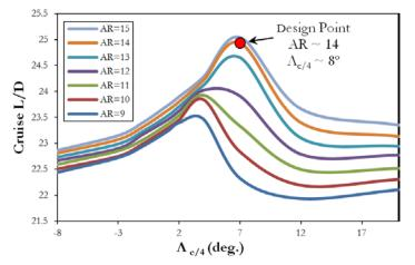
Fig. 17 Parametric study of cruise L/D vs. quarter chord sweep of the wing at various aspect ratios. Design point optimal at AR ~ 14 and  $\Lambda_{c/4}$  ~7-8°.
