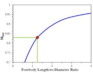
optimal bluntness ratio that minimizes wave drag Fig. 11 Drag Divergence Mach Number vs. Forebody L/D penalties on the forebody, the results of which can be seen in Fig. 12. Efforts were spent to maximize the symmetry of the side profile of the forebody, thus maximizing the extent of NLF<sup>24</sup>. A three dimensional CFD analysis was conducted in order to investigate the extent of laminar flow on the final forebody geometry, the result of which can be seen in Fig. 13.
