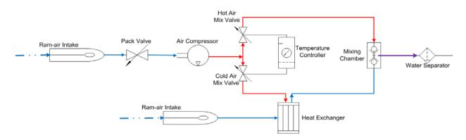
Fig. 46 Air conditioning pack flow diagram. Notice that the recirculation/filtration system is not shown here to be concise.
