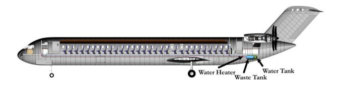
Fig. 54 Inboard profile of Egret featuring water and waste systems along with piping.
