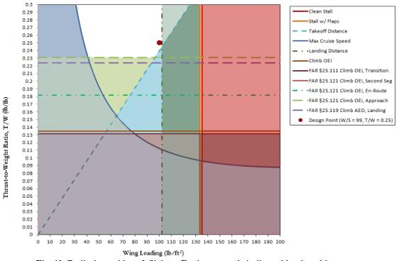
Fig. 10 Preliminary Aircraft Sizing. Design space is indicated by the white area.
