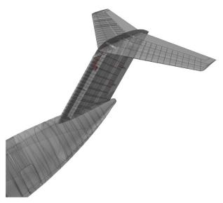
Fig. 7 Empennage and aft body integration of aircraft
