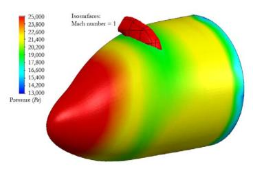
Fig 13 Total pressure contour on the forebody geometry suggests that a favorable pressure gradient is achieved up to the green areas, therefore allowing for possible maintenance of laminar flow. A slight shock is observed on the crown.
