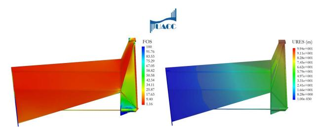
Fig. 35 FEA of aft-mounted engine pylon showing contours of factor of safety (left) and maximum displacement (right)
