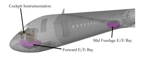
Fig. 51 Location of E/E bays along with Cockpit Instrumentation
