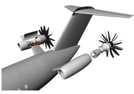
Fig. 44 Engine core detachment
