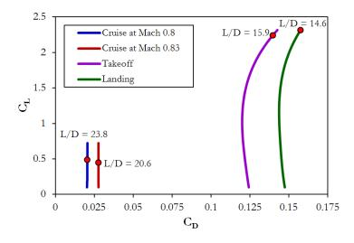
Fig. 23 5<sup>th</sup> order Drag Polars at Cruise, Max Cruise, Takeoff, and Landing Conditions.
