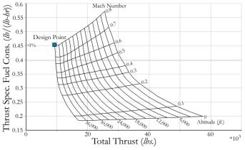
Fig. 32 Engine map used for engine performance analysis. Net thrust of the plane is multiplied by 2 to account for two engines on the Egret
